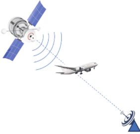
Fig. 3. Forward Scattering Radar System
