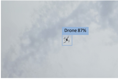
Fig. 9. Detecting a drone at a distance of 30 m from the video camera
