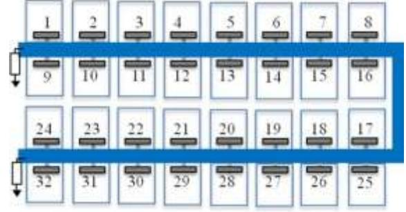
Figure 3: Placement of tilesets with their ID number on the U-shaped transmission line.
